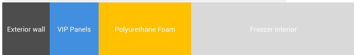
*Figure 2: Sliced diagram of the insulated wall of a freezer*
