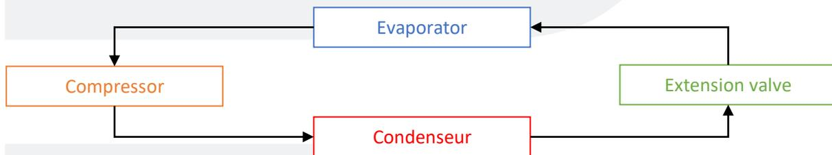
*Figure 1:* Simplified diagram of a refrigeration circuit
