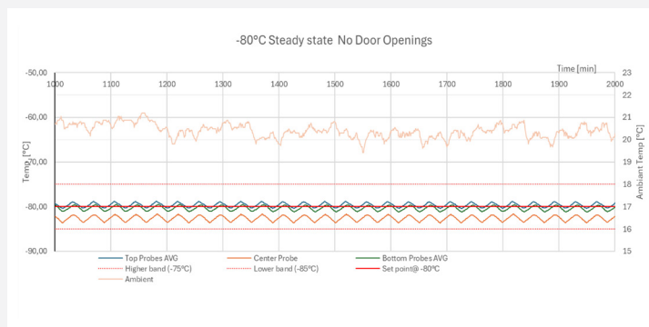
Temperature variation for a setpoint of -80°C for 9 probes.
