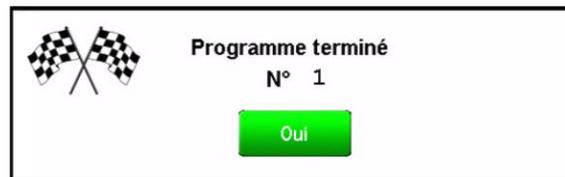
If the user does not click on **Yes**, the machine will continue to regulate the temperature and the airflow according to the instructions of the last line of the program so as not to cause a thermal shock to the DUT.
