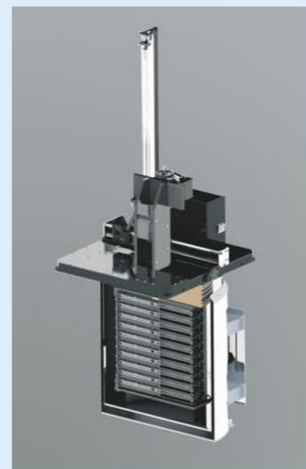
Detail of a disc to store cryotubes inside LN 2 tank
