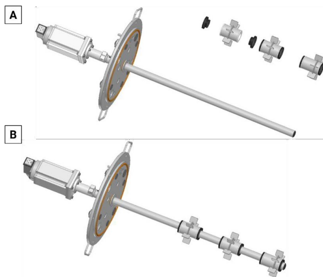
Figure 3.6. Removal of the reactor turbines. A - disassembled turbines and turbine bushings; B - correctly assembled stirrer paddle-type turbines if the turbines rotate counter-clockwise (looking from top of the lid) (for Rushton type turbines turbine rotation direction do not influence mixing quality!).
