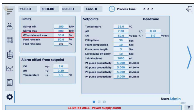
Figure 9.1. Settings for O 2 enrichment
