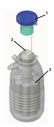
On a clean working surface, in a well ventilated area, warm the unit to ambient temperature. Begin by removing the cap assembly and canister or rack (depending on model), items 1 and 2 shown in Figure.
